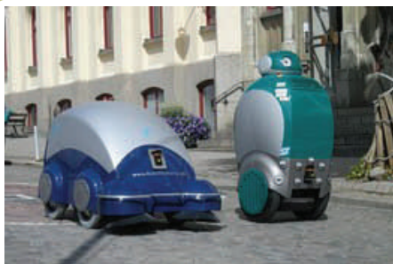
David Zax; The DustClean street sweeper, left, and the DustCart robot, which picks up garbage.
